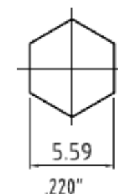
Recommended Crimped Dimensions for Ferrule
