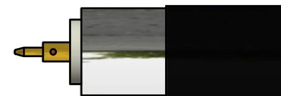
2. Solder Cable Pin to Centre Conductor. Ensure Pin abuts the Insulator. Solder Joint **must** meet IPC-620 Standards.
